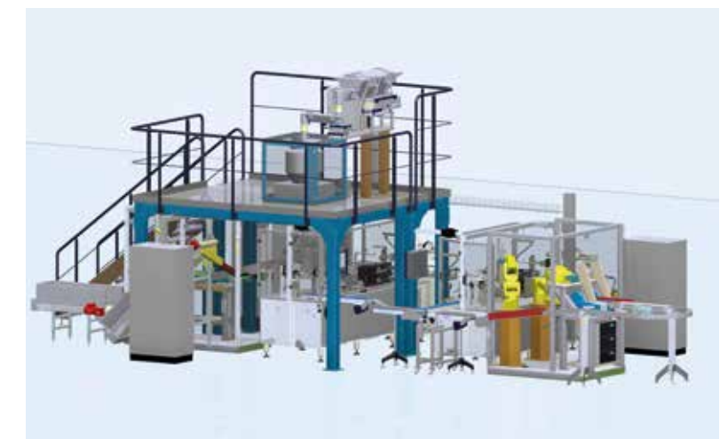
Turn-key project of a packaging line: • 2 horizontal FFS machines • 1 multi head weigher for dosing of piece goods • 4 robots for flexible product handling
