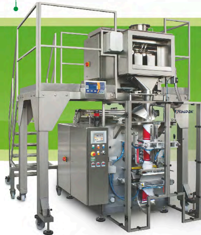
VFF&S Bagger with Zipper Applicator and Radpak Multi Head Weigher.
