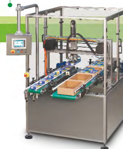
Radpak automatic manipulator-robot with 2-axis motion.
